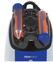
50 mL conical tubes x 2 (horizontally mounted)
