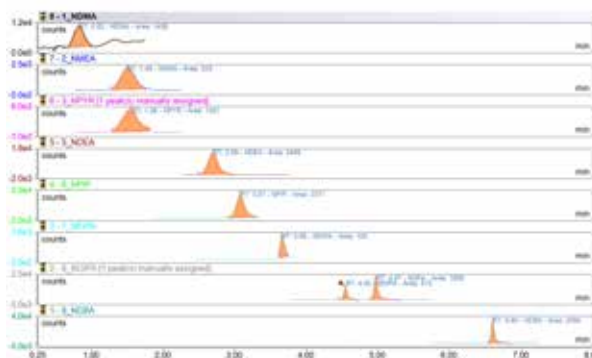
Figure 1. XIC of quantitation ion of nitrosamine impurities in 0.5 ng/mL check standard at a mass tolerance setting of 3 ppm
